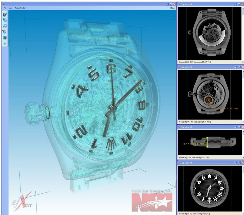
The efX CT software has fast reconstruction and real-time volume/surface rendering with measurement capabilities. Source: North Star Imaging
